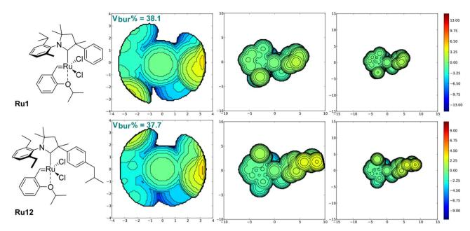
Fig. 3  $V_{bur}$ % steric parameters and maps calculated in SambVca software for CAAC ligands in complexes **Ru1** and **Ru12**. Left: Standard radii (3.5 Å), centre: enlarged radii (10 Å), right: enlarged radii (15 Å). The structures of the complexes (and not simply the ligands) are shown to enhance the readability.
