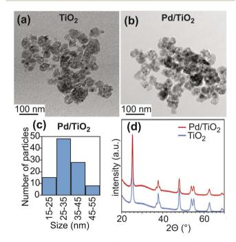
Fig. 2 Properties of  $TiO_2$  and  $Pd/TiO_2$ . Panels (a) and (b) show TEM images for  $TiO_2$  and  $Pd/TiO_2$ . Panel (c) shows a histogram of particle size constructed by counting 100  $Pd/TiO_2$  particles (average particle size 33  $\pm$  8 nm). Panel (d) shows wide-angle PXRD patterns for  $TiO_2$  (blue) and  $Pd/TiO_2$  (red).
