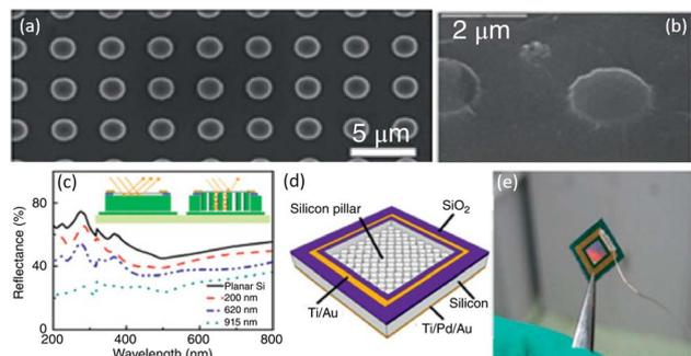
**Fig. 6** SEM image of Si pillar without (a) and with coated graphene (b), (c) the reflectance spectra of Si pillars with different pillar height and planar Si substrate. Inset presents the principle of antireflective effect of Si pillar substrate. (d) Schematic presentation of a G/Si pillar SB-SCs. (e) Photograph of a G/Si pillar SC with junction area of  $0.09 \text{ cm}^2$ . (a)–(e) have been reproduced from 72 with permission from American Institute of Physics.
