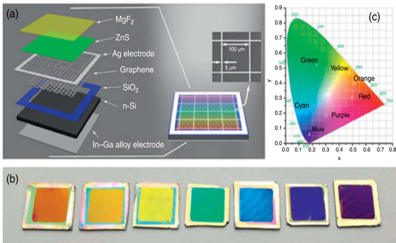
Fig. 9 G/Si SB-SCs with (a) schematic presentation of the color device, (b) photographs of device area:  $1 \text{ cm}^2$  with various colors, and (c) coordinates of seven colors in CIE chromaticity. (a) and (b) Has been reproduced from ref. 99 with permission Elsevier.
