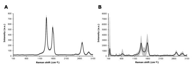
Fig. 3 Raman spectra of (A) the MWCNT coating and (B) the MWCNT/TiO<sub>2</sub> coating, where the black line presents an average Raman spectrum and the gray area is a standard deviation of the signal.
