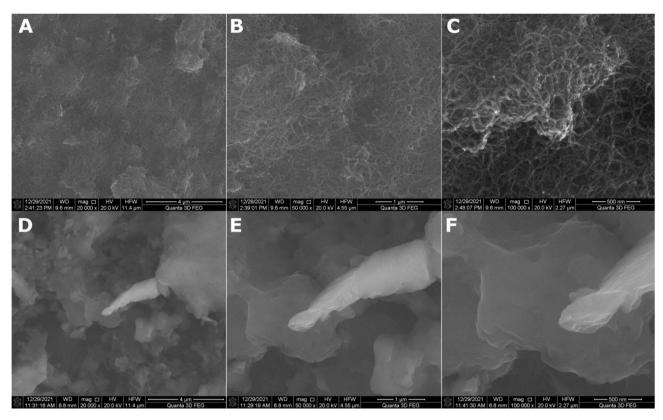
Fig. 2 SEM surface topography of the MWCNT coating (A-C) and the MWCNT/TiO<sub>2</sub> coating (D-F) demonstrated in different resolutions.
