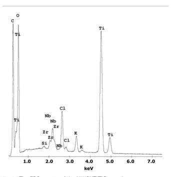
Fig. 1 The EDS spectra of the MWCNT/TiO<sub>2</sub> coating.
