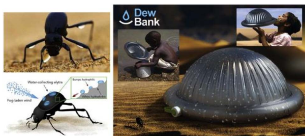
Fig. 18 Dew bottle, inspired by the method of water absorption in the structure of the Namib beetle. Reproduced from ref. 75 with permission from Renewable and Sustainable Energy Reviews .
