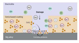
**Fig. 2** Possible self-healing mechanisms of cerium-based coatings. 1. The particles generate a physical blockage of the electrolyte diffusion pathways. 2. Ceria can stabilize the corrosion products of Mg alloys. 3. OH ions can adsorb on the ceria surface, and deposit on the damaged surface. 4. Ceria can adsorb chloride ions.
