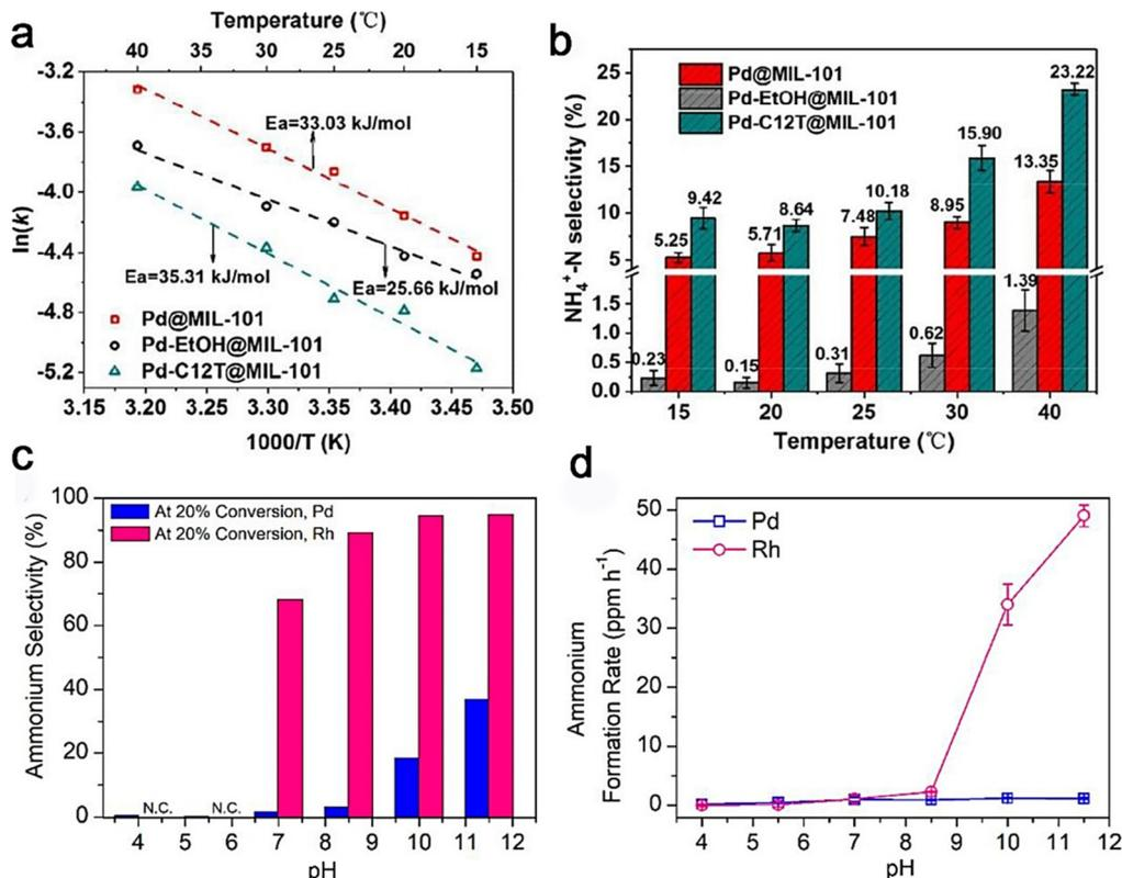
**Fig. 7** (a) Experimental estimation of nitrite reduction activation energies ( $E_a$ ) on different Pd surfaces. (b) Effects of the reaction temperature on ammonia selectivity on various Pd surfaces.<sup>38</sup> Copyright 2018, the Royal Society of Chemistry. (c and d) Effects of varying pH values on the selectivity of ammonia and the ammonia production rates on Pd and Rh.<sup>87</sup> Copyright 2019, American Chemical Society.
