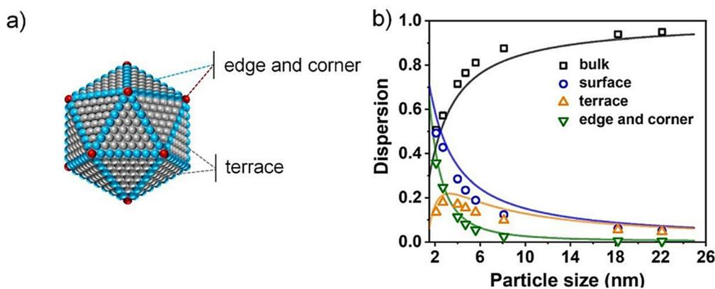
**Fig. 4** (a) Schematic diagram of a structurally stable icosahedral Pd NP. (b) The ratio of bulk, surface, terrace, edge, and corner atoms on icosahedral Pd NPs with different sizes.<sup>72</sup> Copyright 2020, the Royal Society of Chemistry.
