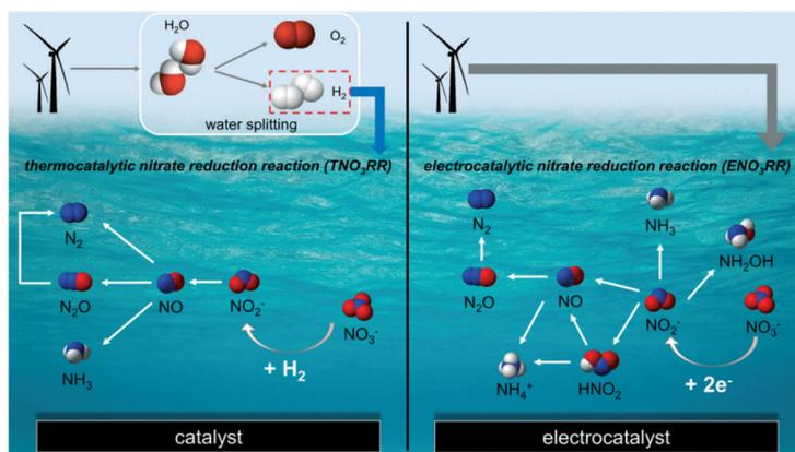
**Fig. 13** Simplified reaction mechanism of the thermal nitrate reduction reaction (TNO<sub>3</sub>RR) and the electrocatalytic nitrate reduction reaction (ENO<sub>3</sub>RR).<sup>146</sup> Copyright 2018, the Royal Society of Chemistry.
