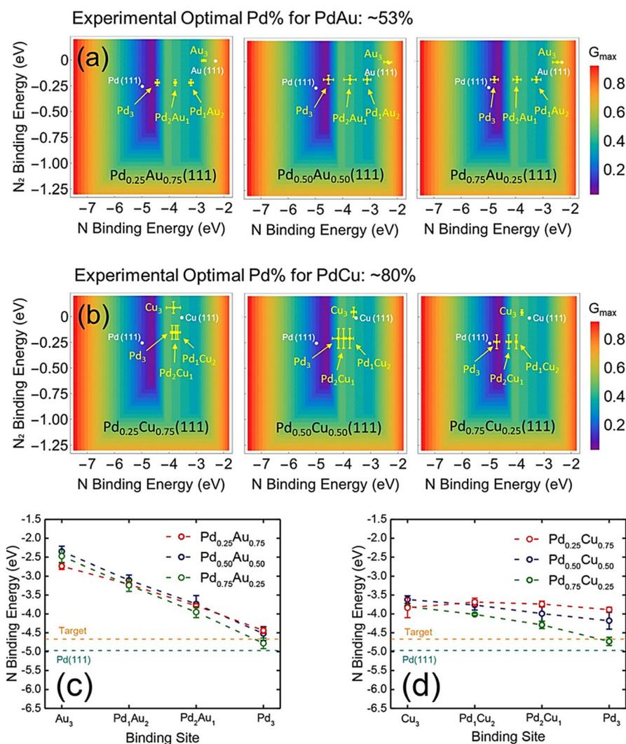
**Fig. 10** (a and b) Predictions of thermal nitrite reduction at triatomic ensembles on PdAu and PdCu alloy surfaces. (c and d) N binding energies at the triatomic ensembles of PdAu and PdCu (111).<sup>36</sup> Copyright 2019, American Chemical Society.
