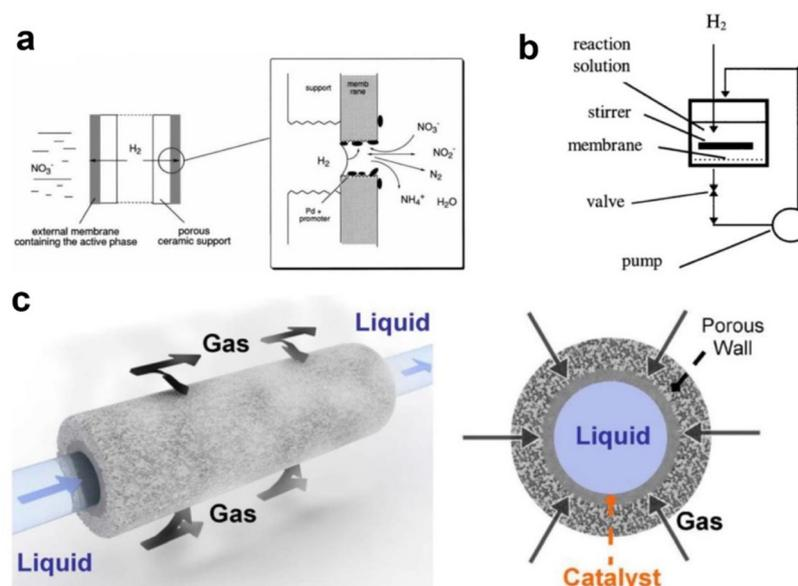
**Fig. 2** (a) Schematic illustration of a catalytic membrane reactor for nitrate and nitrite reduction. (b) The flow-through configuration of a catalytic membrane reactor.<sup>49</sup> Copyright 2013, American Chemical Society. (c) The gas–liquid–solid contact in a porous ceramic reactor.<sup>50</sup> Copyright 2011, Elsevier.
