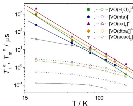
Fig. 5 Temperature dependence of  $T_1^e$  (filled symbols) and  $T_m^e$  (hollow symbols) for the oxovanadium(IV) complexes studied in this work. The solid lines correspond to the fits of the data to a Raman type of relaxation (see the text). Dotted lines are a guide to the eye.
