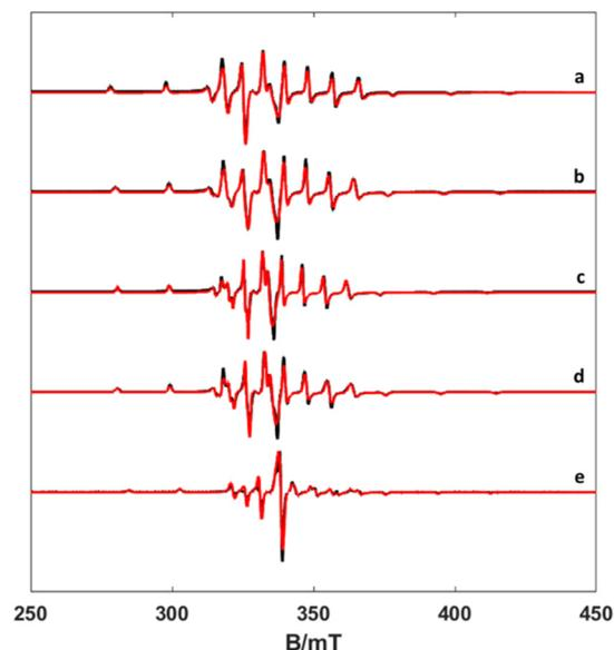
**Fig. 2** X-band CW EPR spectra of frozen solutions of complexes (a) [VO(H<sub>2</sub>O)<sub>5</sub>]<sup>2+</sup>, (b) [VO(nta)(H<sub>2</sub>O)]<sup>-</sup>, (c) [VO(Hdtpa)]<sup>2-</sup>, (d) [VO(ox)<sub>2</sub>(H<sub>2</sub>O)]<sup>2-</sup>, and (e) [VO(acac)<sub>2</sub>(H<sub>2</sub>O)] (experimental black line, simulation red one) at 77 K, 1 mW power and 0.2 mT modulation amplitude.
