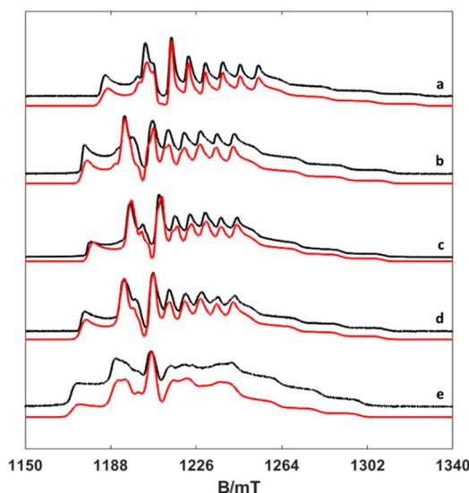
Fig. 4 Experimental (black) and simulated (red) Q-band ESE spectra (a) [VO(H<sub>2</sub>O)<sub>5</sub>]<sup>2+</sup>, (b) [VO(nta)(H<sub>2</sub>O)]<sup>-</sup>, (c) [VO(Hdtpa)]<sup>2-</sup>, (d) [VO(ox)<sub>2</sub>(H<sub>2</sub>O)]<sup>2-</sup>, and (e) [VO(acac)<sub>2</sub>(H<sub>2</sub>O)].
