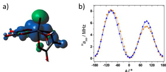
**Fig. 7** Spin density distribution in  $[\text{VO}(\text{oxa})_2(\text{H}_2\text{O})]^{2-}$  calculated at the TPSSh/Def2-TZVPP level. (a) Isosurface of the spin density corresponding to 0.0004 au (positive values in blue). (b)  $^H a_{\text{iso}}$  values calculated for the <sup>1</sup>H nuclei of the coordinated water molecule as a function of  $\phi$  (see the text). The different height of the two maxima is associated with slightly different V–OH<sub>2</sub> distances.
