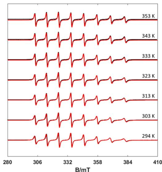
**Fig. 3** Experimental (black) and simulated (red) X-band CW EPR spectra of the [VO(nta)]<sup>-</sup> complex recorded at different temperatures (10 mW power and 0.5 mT modulation amplitude).
