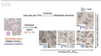
Iodine-influenced morphological evolution of micrometer-sized poly(methyl methacrylate)block-poly(vinyl acetate) particles upon hydrolysis
