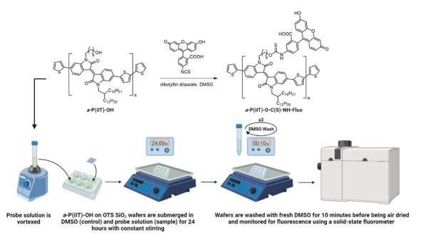
Fig. 5 Schematic of the functionalization of a-P(iIT)-OH (thin film) with fluorescein isothiocyanate (FITC) to afford a-P(iIT)-O-C(S)-NH-Fluo.
