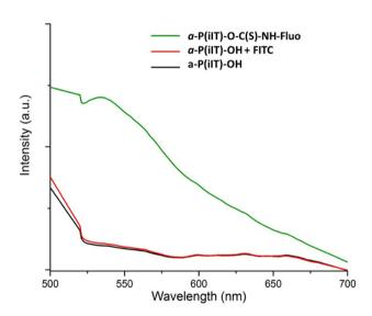
Fig. 6 Fluorescence emission studies for a-P(iIT)-OH (control, black line), a-P(iIT)-OH dipped in fluorescein solution (control, red line) and fluorescein-functionalized a-P(iIT)-O-C(S)-NH-Fluo (green line) thin films on SiO<sub>2</sub> in the solid state. All samples were excited at 495 nm and monitored for fluorescence emission between 500-700 nm.
