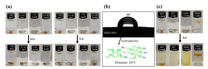
Fig. 8 (a) Digital photo of FDV-1071 in the aqueous solution of HCl and NaOH, (b) water contact angle of FDV-1071 and (c) digital photo of FDV-1071 in 1 M HCl + EtOH (THF) (v:v, 8:2) and in 1 M NaOH + EtOH (THF) (v:v, 8:2).
