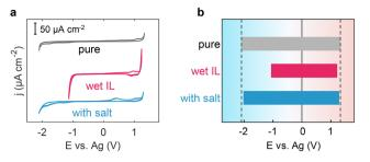
Fig. 5 Electrochemical windows for electrolytes. (a) Cyclic voltammograms of HOPG in pure [Emim][TFSI], wet [Emim][TFSI] and wet [Emim][TFSI] upon adding a salt. Scan rate: 100 mV s<sup>-1</sup>. Electrochemical windows for pure [Emim][TFSI], wet [Emim][TFSI] and wet [Emim][TFSI] upon adding a salt. The cathodic and anodic limits were determined according to a cut-off of  $\pm 30 \, \mu A \, cm^{-2}$ .
