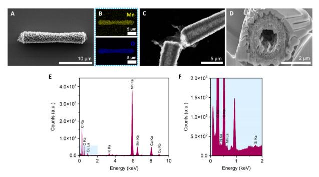
Fig. 4 Characterization of MnO<sub>2</sub>/Lac micromotors. (A) High-resolution FESEM image of a MnO<sub>2</sub> micromotor after the hydrothermal reaction. (B) EDS-mapping of A, showing the Mn (yellow) and O (blue). (C) FETEM image of a MnO<sub>2</sub> micromotor after laccase immobilization. (D) Cross-section of a MnO<sub>2</sub> micromotor. (E) Elemental analysis spectrum of a MnO<sub>2</sub>/Lac micromotor. (F) Magnification of blue square in figure (E) from 0 to 2 keV.
