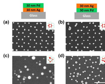
**Fig. 6** SEM images of Pd/Ag/Glass honeycomb array after (a) thermal annealing and (c) applying five  $100 \text{ mJ cm}^{-2}$  pulses. Ag/Pd/Glass honeycomb array after (b) thermal annealing and (d) applying five  $100 \text{ mJ cm}^{-2}$  pulses. The scale bar is  $1 \mu\text{m}$  and applies to all images.
