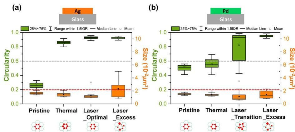
**Fig. 3** Size and circularity distribution of (a) Ag and (b) Pd particles. The pristine, thermally annealed, and laser-treated samples were statistically analyzed. The red dashed line is the circularity of the perfect concave triangle, and the gray dashed line is the circularity of the perfect equilateral triangle. The scheme below the x-axis indicates the morphology and spatial arrangement of the correlated sample.
