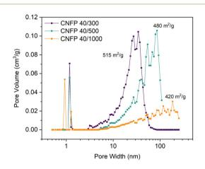
$\begin{tabular}{ll} Fig.~2 & Pore size distributions of CNFPs determined by nitrogen physisorption using the DFT model. \end{tabular}$
