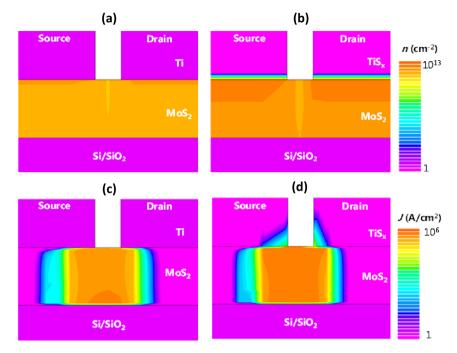
Fig. 6 (a and b) 2D contour plots of the induced charge carrier density and (c and d) current density for Ti and TiS<sub>2</sub> contacts to MoS<sub>2</sub>, respectively. Simulations were performed for 1.2 nm of MoS<sub>2</sub>, 5 nm of Ti and 1.2 nm of TiS<sub>2</sub> at  $V_{DS} = 1$  V and  $V_{GS} = 30$  V.
