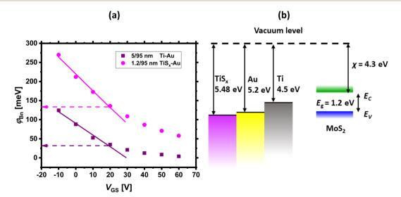
Fig. 5 (a) Effective Schottky barrier height ( $\varphi_{Bn}$ ) as a function of  $V_{GS}$  for both Ti/Au and TiS<sub>x</sub>/Au contacts to MoS<sub>2</sub> FETs. Below the flat band condition,  $\varphi_{Bn}$  reduces linearly with increasing  $V_{GS}$ , which is marked by the fitted straight lines in both contact cases, (b) energy band diagrams of Ti, sulfur-deficient TiS<sub>x</sub><sup>62</sup> and Au with respect to MoS<sub>2</sub>.
