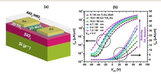
Fig. 1 (a) Schematics of the fabricated MoS<sub>2</sub> FETs, (b) measured transfer curves of the devices with series of TiS<sub>x</sub> contact thicknesses, in both semilog and linear scales. Data for the reference sample is also provided.
