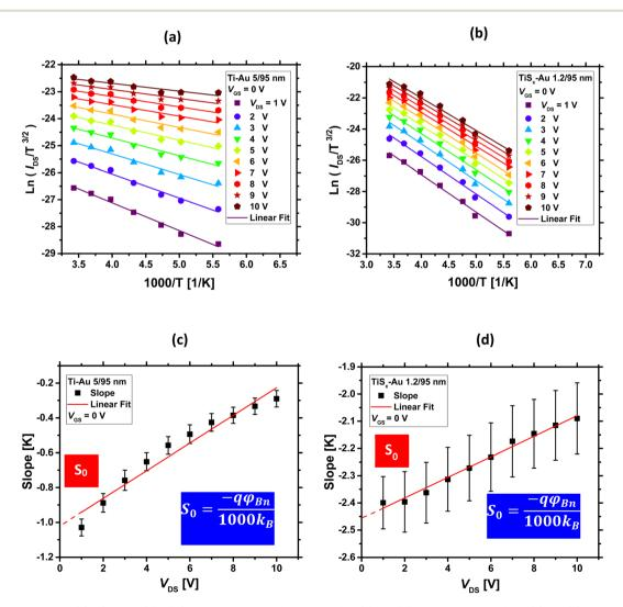
Fig. 4 Arrhenius plots for (a) Ti/Au and (b) TiS<sub>x</sub>/Au contacts to MoS<sub>2</sub> at  $V_{GS} = 0$  V, (c) and (d) extracted slopes from (a) and (b) as a function of  $V_{DS}$ , at  $V_{GS} = 0$  V. The vertical axis-intercept (S<sub>0</sub>) yields  $\varphi_{Bn}$  at  $V_{GS} = 0$  V.
