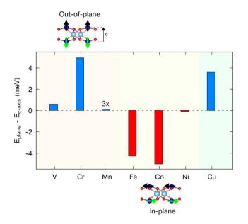
Fig. 4 Magnetocrystalline anisotropy energy of the transition metal ilmenenes. In blue, compounds with out-of-plane anisotropy; in red, with in-plane magnetic moments. For the case of manganese titanate, the magnitude was enhanced by a factor of 3 to make it visible in the shown range.
