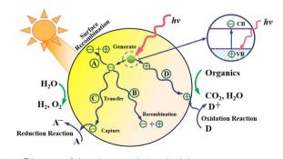
Fig. 1 Diagram of the photocatalytic principle.
