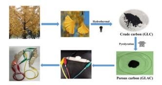
Scheme 1 Synthetic procedure of porous carbon from gingko leaves.
