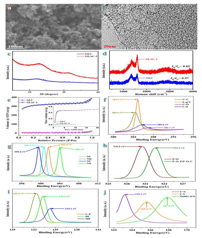
Fig. 1 (a) FESEM image of GLAC-2; (b) TEM image of GLAC-2; (c) XRD patterns of GLC and GLAC-2; (d) Raman spectrum of GLC and GLAC-2; (e)  $N_2$  adsorption/desorption isotherms and the pore size distribution of GLC and GLAC-2; (f) high-resolution C 1s of GLAC-2; (g) high-resolution N 1s of GLAC-2; (h) high-resolution O 2p of GLAC-2; (i) high-resolution P 2p of GLAC-2; (j) high-resolution S 2p of GLAC-2.
