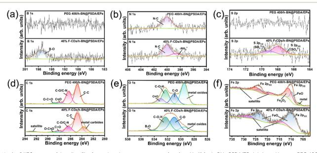
Fig. 10 (a-f) XPS spectra of the tribo-film formed on the worn counter surface (steel ball) for h-BN@PSDA/EPs lubricated by pure PEG 400 and 40 wt% F-CDs in PEG 400
