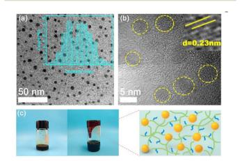
Fig. 2 (a) TEM with low resolution and (b) HR-TEM images of fluid-like carbon dots. The inset in (a) shows the particle size distribution of the solvent-free carbon dot nanofluid identified in yellow. (c) Flow schematic of the solvent-free carbon dot nanofluid and the mechanism of the polymeric three-dimensional network structure.
