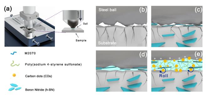
Fig. 11 (a) Schematic of the lubrication mechanism for h-BN@PSDA/EPs lubricated by 40 wt% F-CDs in PEG 400. Schematic of the lubrication mechanism of (b) EP, (c) h-BN@PSDA/EPs, (d) h-BN@PSDA/EPs lubricated by PEG 400, (e) h-BN@PSDA/EPs lubricated by 40 wt% F-CDs in PEG 400
