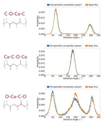
Fig. 4 Angle distributions of key polymer backbone dihedrals of amorphous PLLA in a pyrophyllite composite system.
