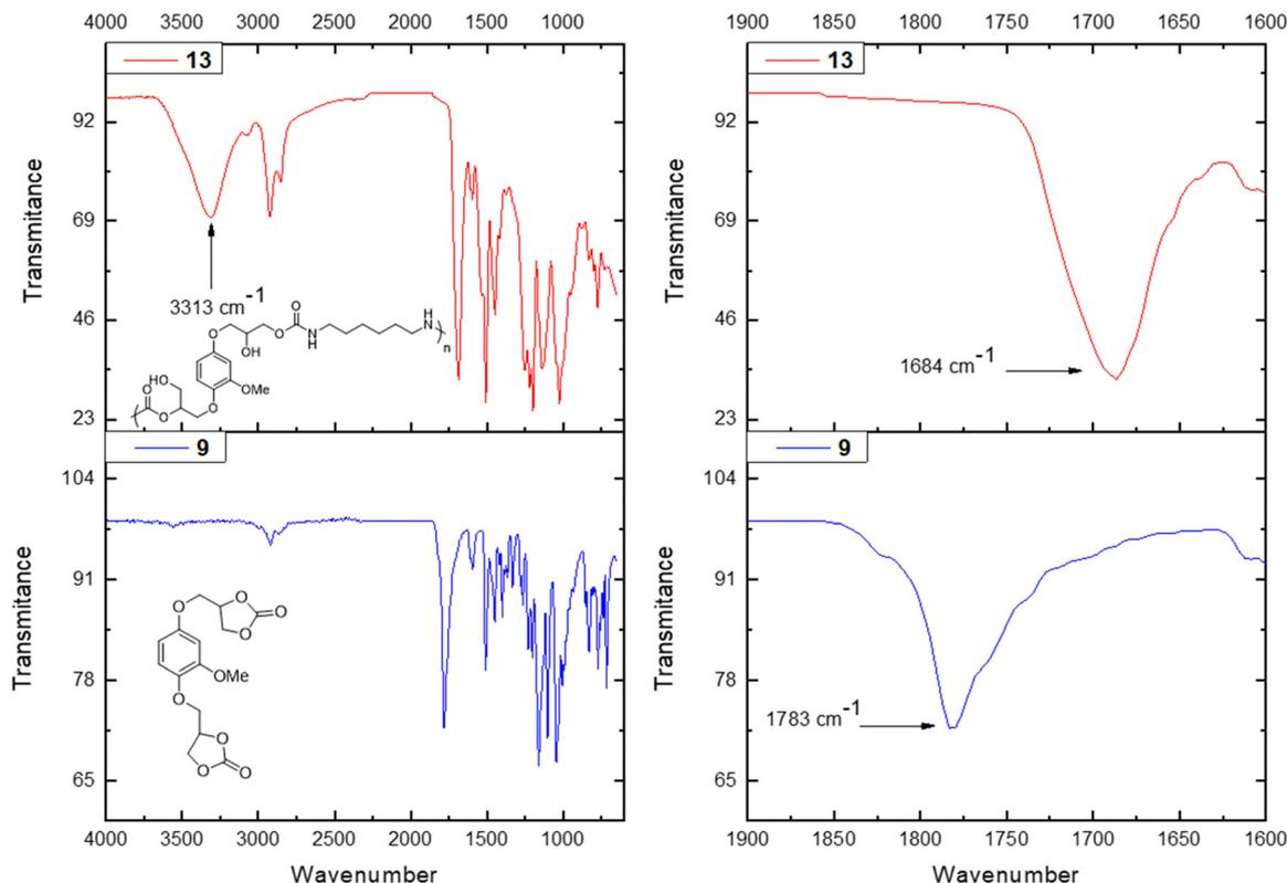
Fig. 1 FT-IR spectrum of hydroquinone-based PHUs (**13**) prepared from hydroquinone-based bis-carbonate (**9**) (left), zoom of carbonyl stretching region of hydroquinone-based PHUs (**13**) prepared from hydroquinone-based bis-carbonate (**9**) (right).
