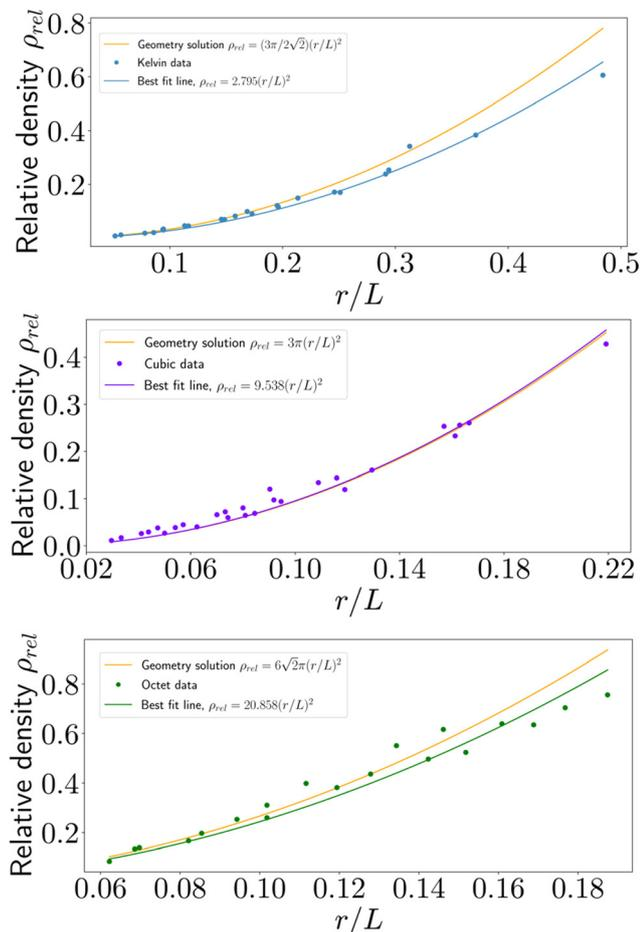
Fig. 2 Empirical relative density relationships as a function of beam aspect ratio,  $r/L$ , for each geometry. The first-order model is also shown for reference, although slight disagreement exists due to double-counting of the nodal intersections, particularly at high relative densities.
