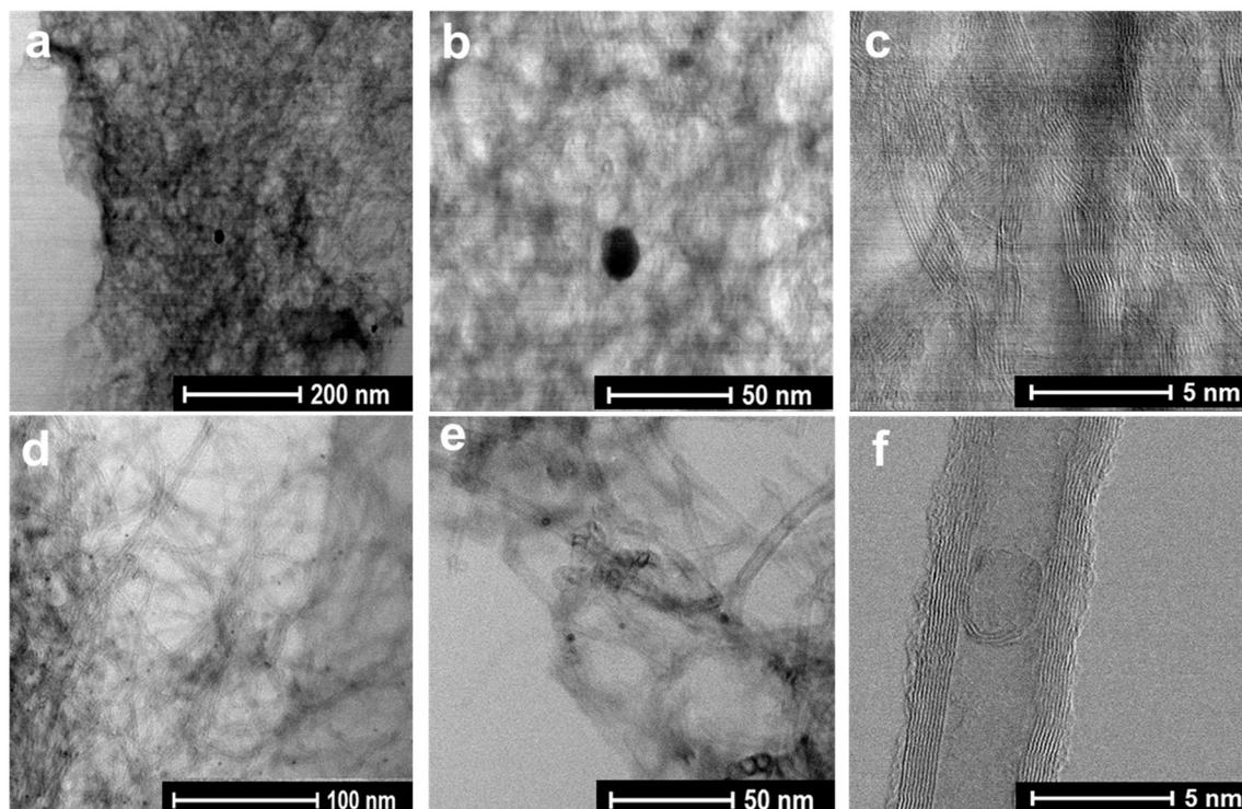
**Fig. 3** BF-STEM images for (a–c) Fe<sub>1</sub>Co<sub>1</sub>-ZNT-900 and (d–f) Fe<sub>1</sub>Co<sub>2</sub>-ZNT-900 catalysts at different resolutions.
