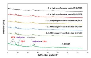
Fig. 10 Changes in the X-ray diffraction (XRD) patterns of the assynthesized and H<sub>2</sub>O<sub>2</sub> treated N-G/MOF samples.
