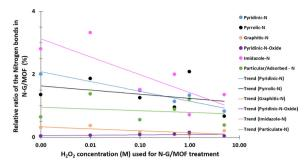
Fig. 7 Changes in the relative ratios of nitrogen (N) bonds of the N-G/ MOF samples with increasing concentration of H<sub>2</sub>O<sub>2</sub> used for the treatments. The data was obtained by the UHV-XPS system and postanalyzed for relative ratios.
