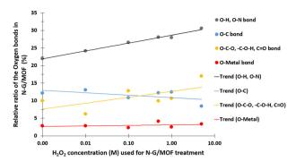
Fig. 9 Changes in the relative ratios of oxygen (O) bonds of the N-G/ MOF samples with increasing concentration of H<sub>2</sub>O<sub>2</sub> used for the treatments. The data was obtained by the UHV-XPS system and postanalyzed for relative ratios.
