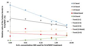
Fig. 5 Changes in the relative ratios of carbon (C) bonds of the N-G/ MOF samples with increasing concentration of H2O2 used for the treatments. The data was obtained by the UHV-XPS system and postanalyzed for relative ratios.
