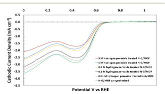
Fig. 2 Electrochemical performance evaluation of the as-synthesized and H<sub>2</sub>O<sub>2</sub> treated N-G/MOF samples in alkaline medium (0.1 M KOH), experimentally taken by the LSV technique of the RDE system.
