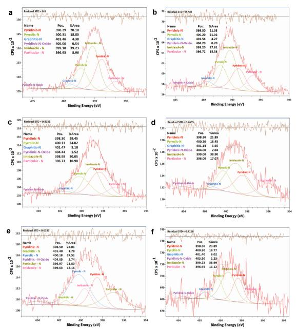
Fig. 6 XPS analyses of the N 1 s narrow scan spectra of N-G/MOF samples: (a) as-synthesized N-G/MOF; (b) 0.01 M; (c) 0.1 M; (d) 0.5 M; (e) 1 M; and (f) 5 M H<sub>2</sub>O<sub>2</sub> treated N-G/MOF.
