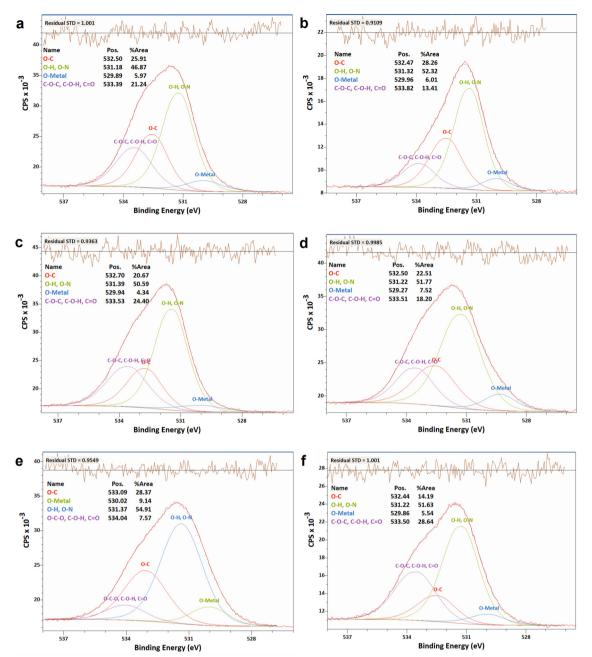
Fig. 8 XPS analyses of the O 1s narrow scan spectra of N-G/MOF samples: (a) as-synthesized N-G/MOF; (b) 0.01 M; (c) 0.1 M; (d) 0.5 M; (e) 1 M; and (f) 5 M H<sub>2</sub>O<sub>2</sub> treated N-G/MOF.
