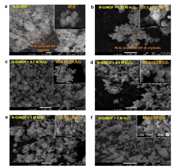
Fig. 12 SEM images of the N-G/MOF samples: (a) as-synthesized N-G/MOF; (b-f) 0.01 M to 5 M H<sub>2</sub>O<sub>2</sub> treated N-G/MOF, gradual material structural fragmentation observed. Insets (a-f): corresponding SEM images of H<sub>2</sub>O<sub>2</sub>-treated ZIF-8 samples.
