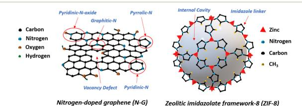
Fig. 1 Schematics of the chemical structures of nitrogen-doped graphene (N-G) and zeolitic imidazolate framework-8 (ZIF-8). The unit cells of ZIF-8 are dodecahedral-shaped; the sphere at the center represents the cavity created by the framework.
