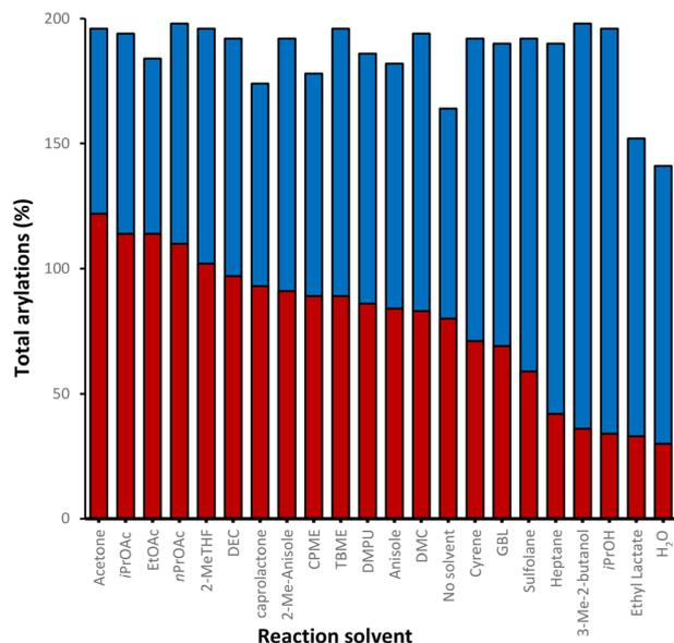
**Scheme 2** Screen of green solvents at different reaction times. Yields were measured by GC-FID analysis of the crude reaction mixture using hexadecane as the internal standard. Solvent acronyms can be found in endnotes.<sup>46</sup>
