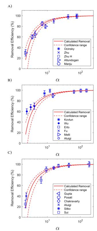
Fig. 3 Removal efficiency (%) as a function of parameter  $\alpha = Q_m K_L M/V$ : the experimental points from the literature are compared to the expected behaviour of eqn (6) (red line). Upper and lower confidence ranges, calculated by assuming a 20% relative error in the determination of  $\alpha$ , are shown as red dotted lines. The experimental points are from papers reported in Table 1. Different adsorbates were considered: (A) arsenic. (B) Organic molecules and (C) other heavy metals.
