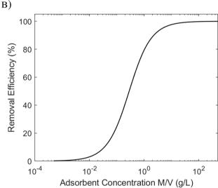
**Fig. 2** (A) Removal efficiency (%) as a function of initial concentration of adsorbed molecules, showing also a common numerical value of low concentration (5 ppm, magenta dotted line) and the low concentration limit,  $1/K_{\rm L}=15$  ppm (black dotted line). (B) Removal efficiency (%) as a function of adsorbent concentration.
