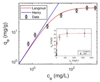
Fig. 1 Adsorption isotherm with Langmuir fit, plotted in logarithmic scale (log-log plot),  $Q_{\rm m} = 63.0 \text{ mg g}^{-1}$ ,  $K_{\rm L} = 65.2 \text{ mL mg}^{-1}$ , V = 25 mL, M = 50 mg. Inset: Isotherm plot in linear scale.
