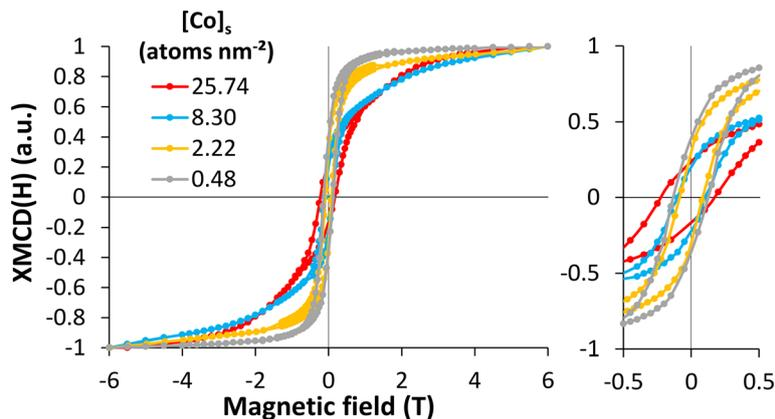
**Fig. 3** XMCD magnetization versus magnetic field measurement at the Co  $L_3$ -edge at 4.2 K for four solid cobalt concentrations (from 0.48 to 25.74 atom per  $\text{nm}^2$ ). All the curves were normalized to 1 in order to compare the magnetization behavior versus the  $[\text{Co}]_s$ . The raw XMCD magnetization curves can be seen in the ESI† (see Fig. S7).
