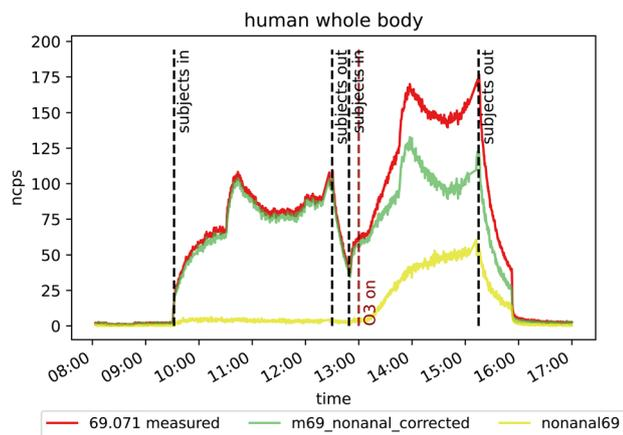
Fig. 3 Signals of measured  $m/z$  69.07 (red), calculated  $m/z$  69.07 from nonanal (yellow) and  $m/z$  69.07 corrected by the contribution of nonanal (green) from the ICHEAR whole body experiment (dermal and breath emission).
