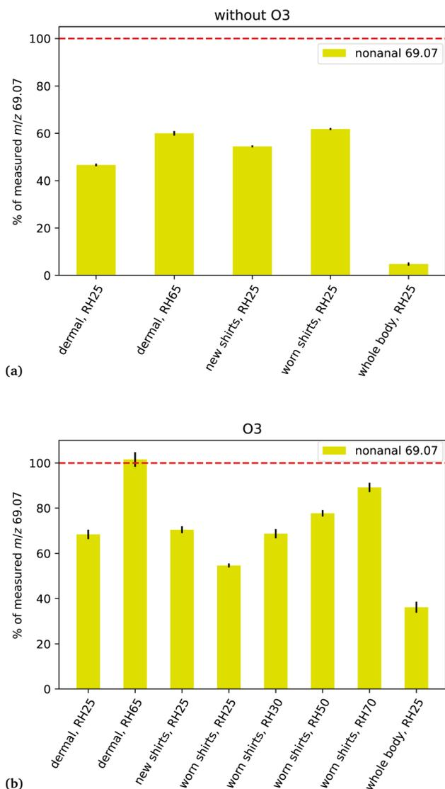
Fig. 2 For different ICHEAR experiments (see Table 2), the yellow bars indicate the percent of the total measured signal for  $m/z$  69.07 due to nonanal as calculated using eqn (3). (a) In the absence of ozone; (b) in the presence of ozone. The small black lines indicate the standard deviation.
