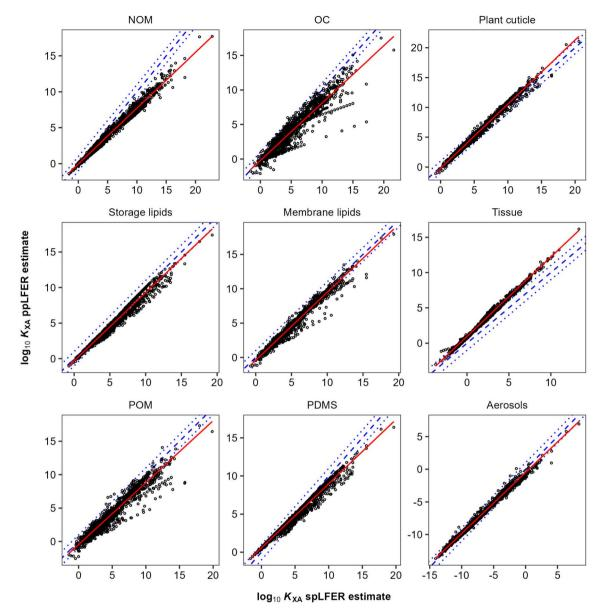
Fig. 1 Correlation between  $\log_{10} K_{XA}$  predicted using system specific ppLFERs plotted against  $\log_{10} K_{XA}$  predicted using spLFERs using  $\log_{10} K_{OA}$ . The red solid lines show the line of best fit, blue dashed lines indicate a 1:1 relationship, and blue dotted lines have slopes of 1 and intercepts of  $\pm 1 \log_{10}$  unit. NOM: natural organic matter; OC: organic carbon; POM: polyoxymethylene; PDMS: polydimethyl siloxane; PUF: polyurethane foam.
