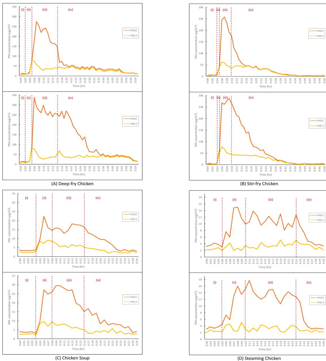
**Fig. 2** Particulate matter emissions during the cooking process of four cooking episode. (A) Deep-fry chicken, (B) stir-fry chicken, (C) chicken soup and (D) steaming chicken, with extractors (upper image) on and (lower image) off. Four stages of cooking process: (i) the background level; (ii) heating of the pot or pan and the oil or water (iii) the main cooking processes; (iv) the post-cooking decay after the end of the entire cooking process.
