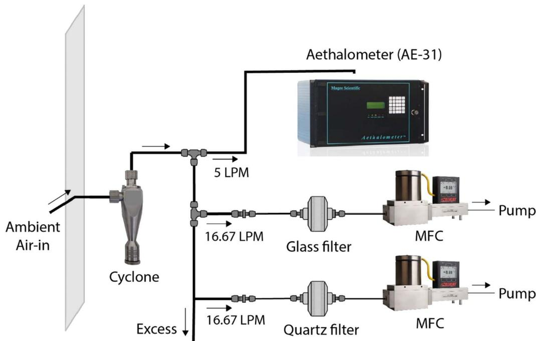
Fig. 1 Sampling set-up used for collecting ambient particulates on glass and quartz-fiber filters. An aethalometer (AE-31) parallelly measured BC for training filter  $R$  to BC model and to validate image-based BC. A cyclone was used at the collective inlet to allow only  $PM_{2.5}$  during sampling.
