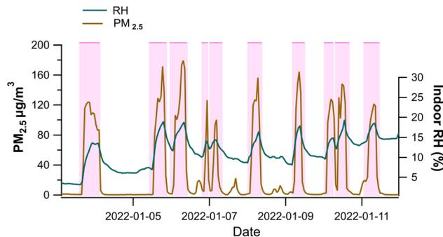
Fig. 8 Effect of humidifier on indoor PM<sub>2.5</sub> emission. Data from one sensor is shown here as a case study.
