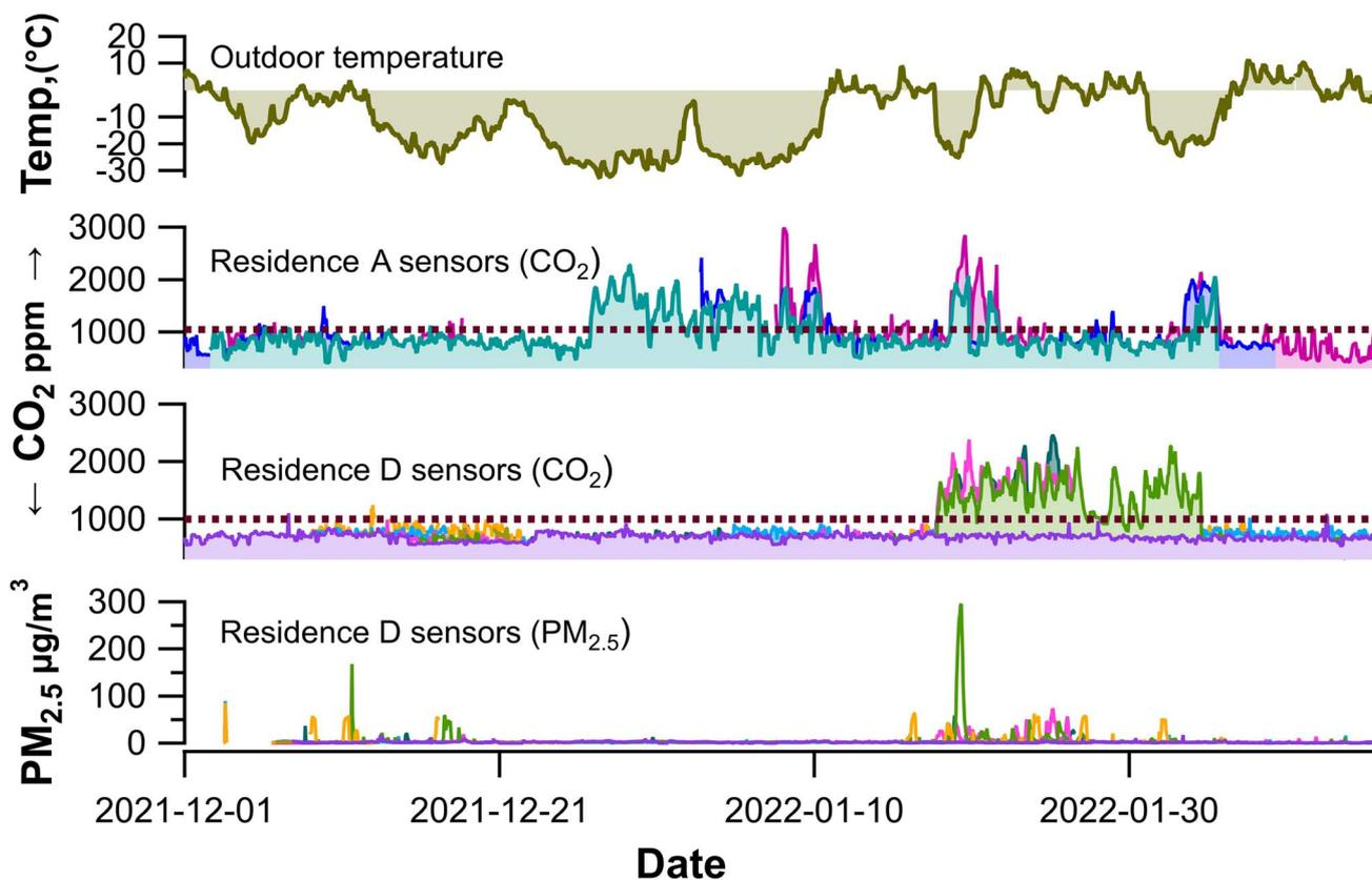
Fig. 11 Impact of outdoor temperature and ventilation on indoor pollutants  $\text{CO}_2$  and  $\text{PM}_{2.5}$  concentration. Impact of outdoor temperature and ventilation on indoor pollutants ( $\text{CO}_2$  and  $\text{PM}_{2.5}$ ) concentration.
