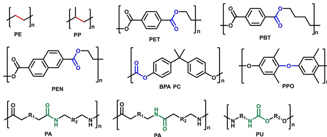
Fig. 1 Different types of plastics for hydroconversion processes.
