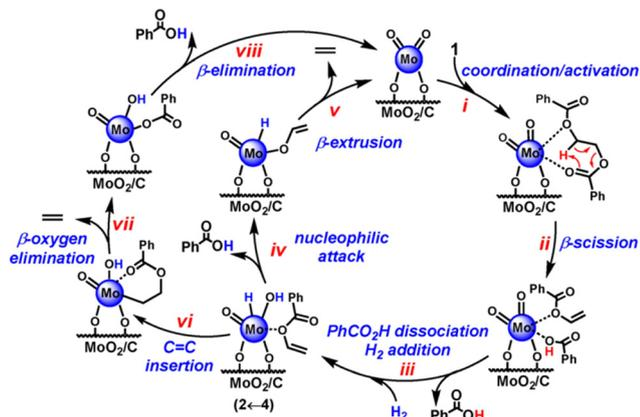
Fig. 10 The mechanism for the hydrogenolysis of PET over the C/MoO<sub>2</sub> catalyst. Reproduced from ref. 82 with permission from Wiley.
