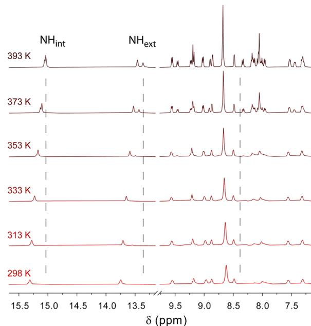
Fig. 3 Variable temperature <sup>1</sup>H NMR spectroscopy of a **C<sub>3</sub>Pyr/C<sub>3</sub>NDI** (1/1) mixture in TCE-*d*<sub>2</sub> ([**C<sub>3</sub>Pyr**] = [**C<sub>3</sub>NDI**] = 5.2 mM).
