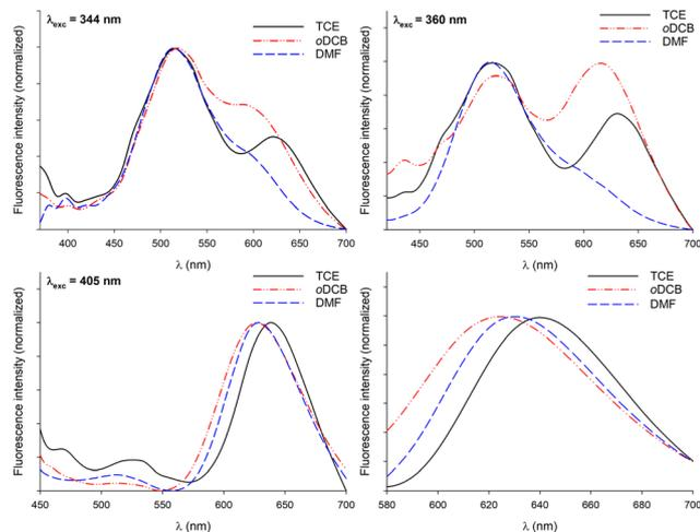
Fig. 8 Normalized emission spectra of  $C_3Pyr/C_3NDI$  (1:1) organogels ( $C = CGC$ ) upon excitation at different wavelengths (bottom right corner: irradiations at  $\lambda_{exc} = 525$  (TCE), 512 (oDCB) and 523 nm (DMF)).
