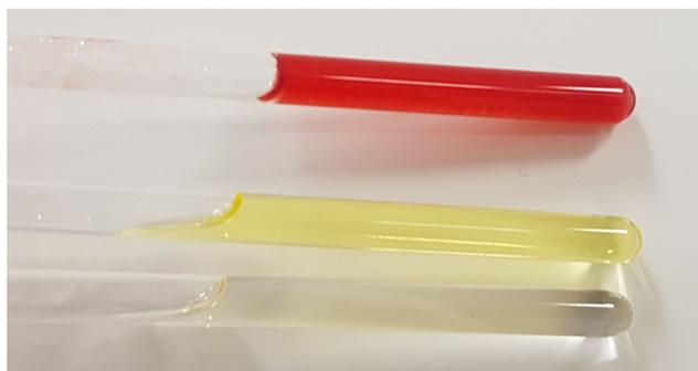
Fig. 2 Top. Donor-acceptor organogel obtained from **C<sub>3</sub>Pyr** and **C<sub>3</sub>NDI** in TCE-*d*<sub>2</sub> ([**C<sub>3</sub>Pyr**] = [**C<sub>3</sub>NDI**] = 5.2 mM). Middle. Solution of **C<sub>3</sub>NDI** in TCE (5.2 mM). Bottom. Solution of **C<sub>3</sub>Pyr** in TCE (5.2 mM).
