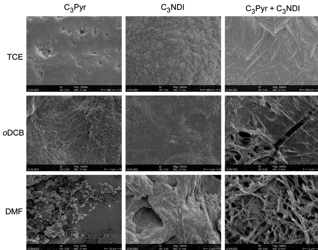
Fig. 6 SEM micrographs of samples prepared by gel deposition of the individual compounds  $C_3$ Pyr (8 mg mL<sup>-1</sup>, a),  $C_3$ NDI (10 mg mL<sup>-1</sup>, b) and their equimolar mixture  $C_3$ Pyr/ $C_3$ NDI (identical concentrations, c) in TCE.
