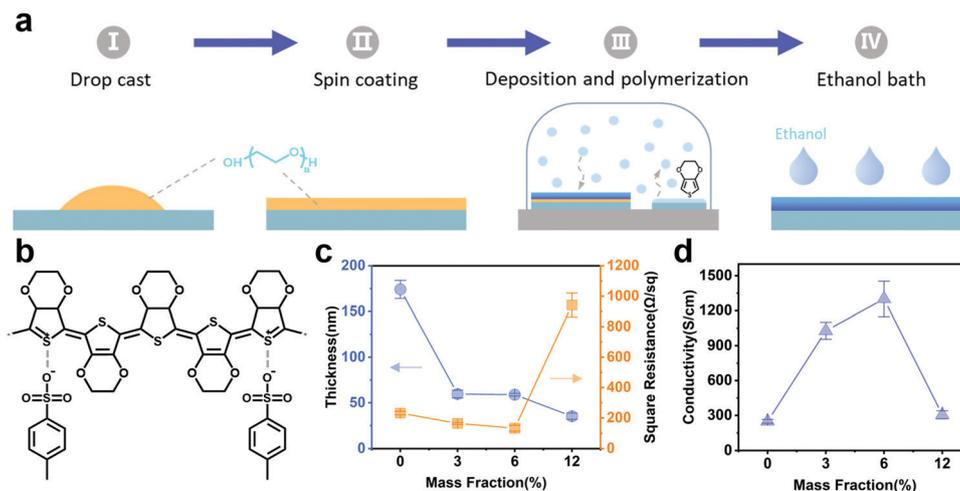
Fig. 1 Synthesis process and conductivity of the VPP PEDOT films. (a) Process flow for the preparing VPP PEDOT film *via* VPP: (I) oxidant dropwise, (II) spin coating, (III) substrate transfer and monomer deposition, (IV) ethanol bath. (b) Chemical structure of VPP PEDOT. (c and d) Thickness and square resistance and conductivity of VPP PEDOT Film with 0, 3, 6, 12 wt% PEG addition.
