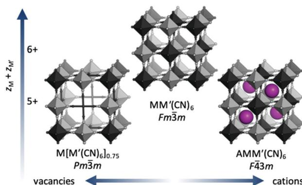
Fig. 1 The crystal structure of Prussian blue analogues. If the charges of the transition metals ( $z_M + z_{M'}$ ) sum to 6, the ordered  $MM'(CN)_6$  is formed. For lower charges, vacancies or A-site cations are included to give the formulae  $M[M'(CN)_6]_{y < 1}$  and  $A_{x > 0}M[M'(CN)_6]$ , respectively.  $M$  is shown in dark grey,  $M'$  in light grey and  $A$  in purple.
