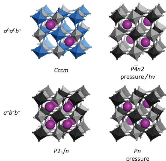
Fig. 5 Tilted structures of Rb-based PBAs. (a)  $\text{Rb}_{0.90}\text{Cu}[\text{Co}(\text{CN})_6]_{0.92}$ , where the tilting is driven by Jahn–Teller distorted Cu (blue) and the unusual Rb arrangement;<sup>26</sup> (b)  $\text{Rb}_{0.97}\text{Mn}[\text{Fe}(\text{CN})_6]_{0.99}$  under pressure;<sup>50</sup> (c)  $\text{Rb}_2\text{MnMn}(\text{CN})_6$  at ambient conditions;<sup>47</sup> and (d)  $\text{Rb}_{0.87}\text{Mn}[\text{Co}(\text{CN})_6]_{0.91}$  under pressure.<sup>49</sup>
