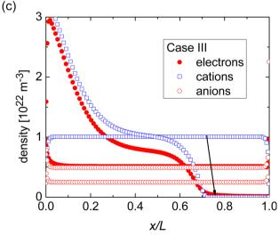
Fig. 2 Simulated profiles of the electron, cation, and anion densities for Cases I, II, and III. The arrows indicate how the density profiles change from before to after the application of the bias voltage stress.
