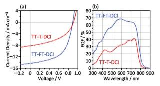
Fig. 6 (a) J-V curves and (b) EQE spectra for PBDB-T:TT-FT-DCI and PBDB-T:TT-T-DCI OSC devices.
