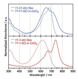
Fig. 5 UV-vis absorption spectra of films (solid lines) and in CHCl<sub>3</sub> solutions (dotted lines) for TT-FT-DCI and TT-T-DCI.
