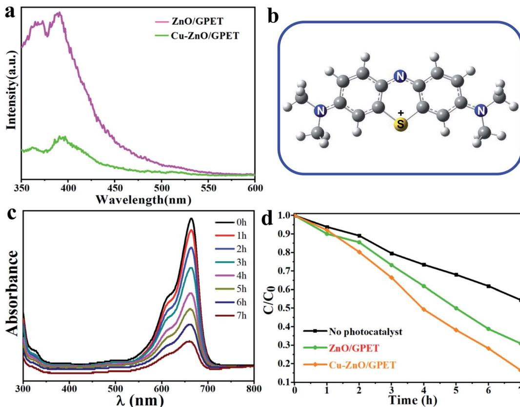
Fig. 3 (a) PL spectra of the Cu<sub>1</sub>-ZnO/GPET composite. (b) Schematic structure of MB<sup>+</sup> cation (optimized by using PBE/6-31G with Gaussian program). (c) Temporal evolution of the UV-vis absorption spectrum in accord with MB of Cu<sub>1</sub>-ZnO/GPET. (d) Photodegradation rate of MB stimulated by UV of samples.
