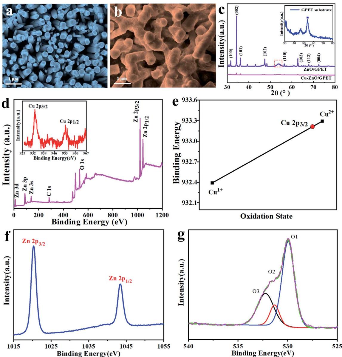
Fig. 1 The FESEM images of (a) ZnO/GPET and (b)  $\text{Cu}_1\text{-ZnO/GPET}$ . (c) The XRD patterns of ZnO/GPET and  $\text{Cu}_1\text{-ZnO/GPET}$  nanomaterials, where inset shows GPET substrate peaks. (d) XPS spectra for  $\text{Cu}_1\text{-ZnO/GPET}$  films and the inset shows Cu 2p peaks. (e) The binding energy of Cu  $2p_{3/2}$  with +2 and +1 oxidation states, respectively. (f and g) High resolution XPS scan of Zn 2p and O 1s for  $\text{Cu}_1\text{-ZnO/GPET}$ .
