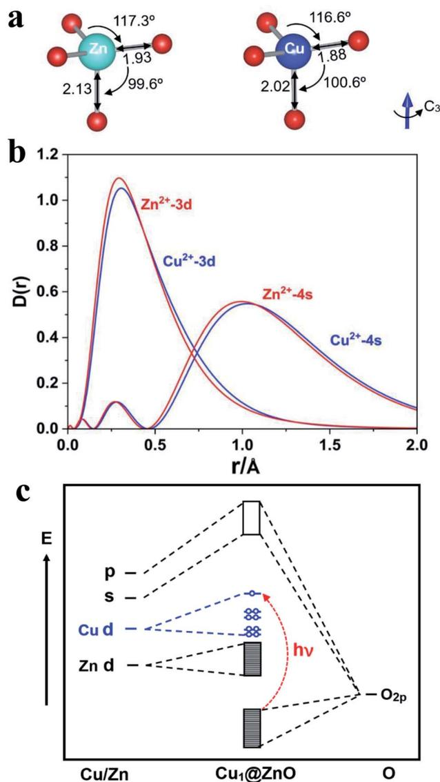
Fig. 6 (a) The local  $C_{3v}$  ligand field of ZnO and doped  $Cu_1@ZnO$  surface in crystal (color code: Cu-blue, O-red, Zn-green). (b) The radial distribution probability density ( $D(r) = r^2 R(r)^2$ ) of atomic orbitals (AOs) of Zn(II) and Cu(II); (c) schematic energy levels of the  $Cu_1@ZnO$  single-atom catalyst.
