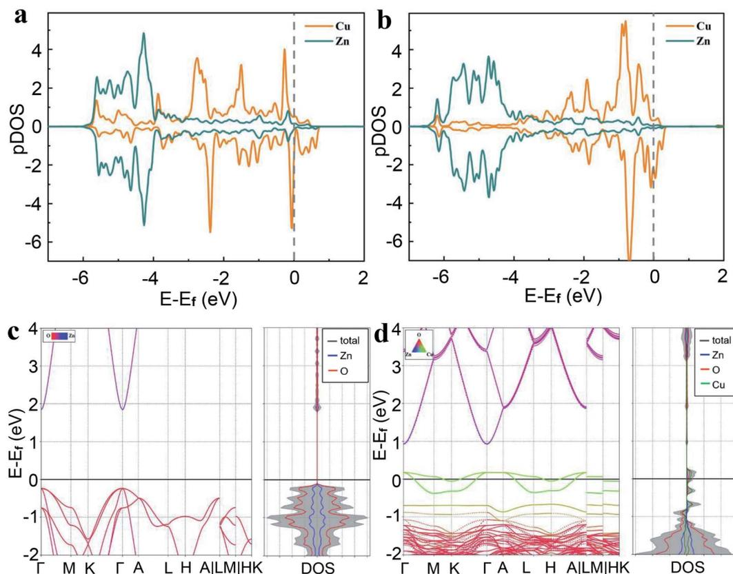
Fig. 5 Projected density of state (pDOS) of surface Zn and Cu atoms in (a) doped  $\text{Cu}_1\text{@ZnO}$  model (Fig. 4b), and (b) supported  $\text{Cu}_1/\text{ZnO}$  model (Fig. 4c). Band structure of (c) pure ZnO and (d) doped  $\text{Cu}_1\text{@ZnO}$  in which one Zn atom in the  $2 \times 2 \times 2$  supercell of ZnO is replaced by one Cu atom.
