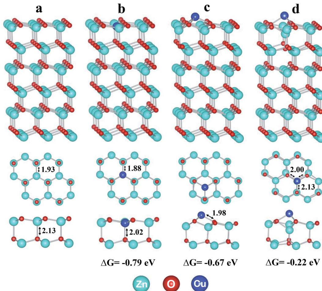
Fig. 4 The optimized structures of (a) pure ZnO, (b) doped Cu<sub>1</sub>@ZnO, and (c and d) supported Cu<sub>1</sub>/ZnO. The formation Gibbs free energies of doped and supported Cu<sub>1</sub> are calculated at 298.15 K and 1 atm. The blue, cyan, and red spheres represent Cu, Zn, and O, respectively.
