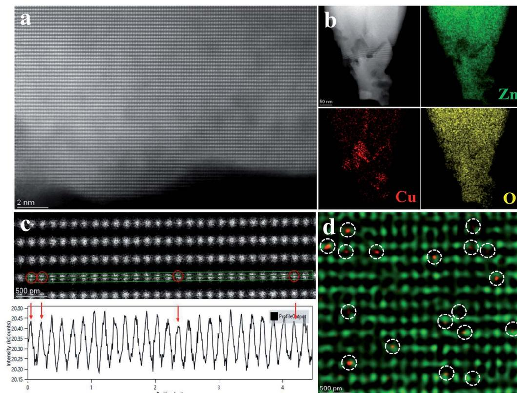
Fig. 2 (a) TEM images for  $Cu$ -ZnO. (b) STEM-EDS elemental mapping of  $Cu$ -ZnO. (c) Line intensity distribution diagram of Cu atoms. (d) HAADF-STEM image of  $Cu_1$ -ZnO. The representative Cu single atom ( $Cu_1$ ) is indicated by the white circle.
