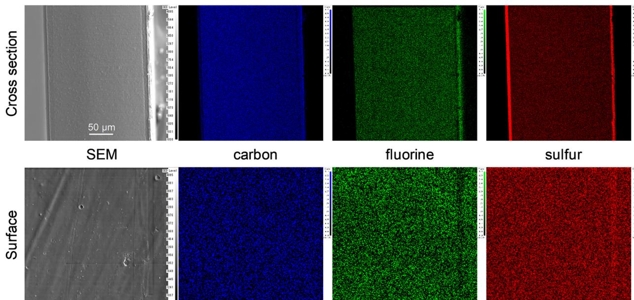
**Fig. 4** SEM and EPMA element mapping images (blue: carbon, green: fluorine, and red: sulfur) of cross section and surface of the ionic SMP gel sensor with PEDOT:PSS electrodes on both surfaces of the gel ( $W_{\text{L}} = 25$  wt%).
