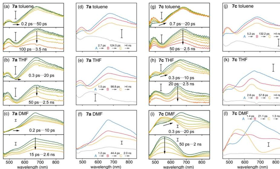
Fig. 5 Transient absorption spectra (a–c and g–i) and species-associated spectra (SAS) (d–f and j–l) of **7a** and **7c** in toluene (upper panel), THF (medium panel) and DMF (lower panel). Time constants were obtained from target analysis with a four step sequential model. The scale bar of signal intensity represents 1 MOD.
