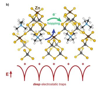
Scheme 2 Conduction pathways for the band-type Fe (a) *versus* hopping-type Zn (b) analogues.
