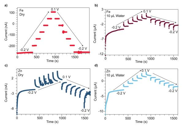
Fig. 1 Chronoamperometry traces of  $TMA_2FeGe_4S_{10}$  and  $TMA_2ZnGe_4S_{10}$  pressed-pellets under applied voltages spanning -0.2 V to 0.1 V when dry (a and c), and after treatment with  $10~\mu$ L of deionized water (b and d), respectively.
