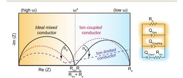
Scheme 3 Generalized impedance response for an ideal mixed conductor (black solid trace), an ion-coupled conductor (dotted red trace; TMA2ZnGe4S10), and ion-limited conductor (dotted blue trace; TMA<sub>2</sub>FeGe<sub>4</sub>S<sub>10</sub>).
