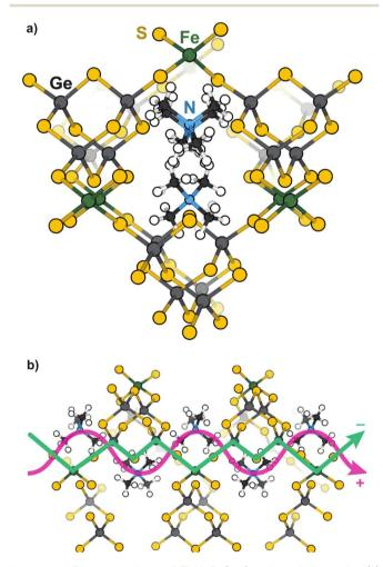
Scheme 1 Representations of  $TMA_2FeGe_4S_{10}$  viewed along the (a) [100] and (b) [101] directions. Proposed conduction pathways of delocalized electrons and extra-framework cations are highlighted in green and pink, respectively.
