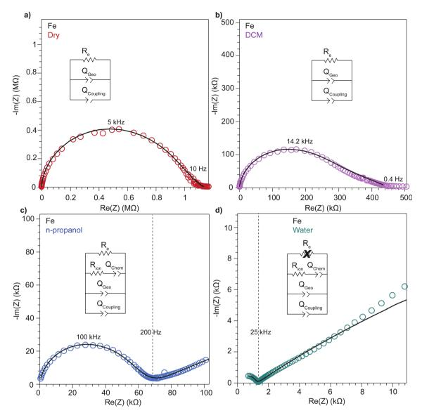
Fig. 3 Nyquist plots of  $TMA_2FeGe_4S_{10}$  pressed-pellets when dry (a) and after addition of DCM (b), n-propanol (c), and deionized water (d). Black traces represent fits to the equivalent circuit diagrams shown in the figure. Crossed-out circuit elements denote elements that are too large to adequately fit to the impedance response
