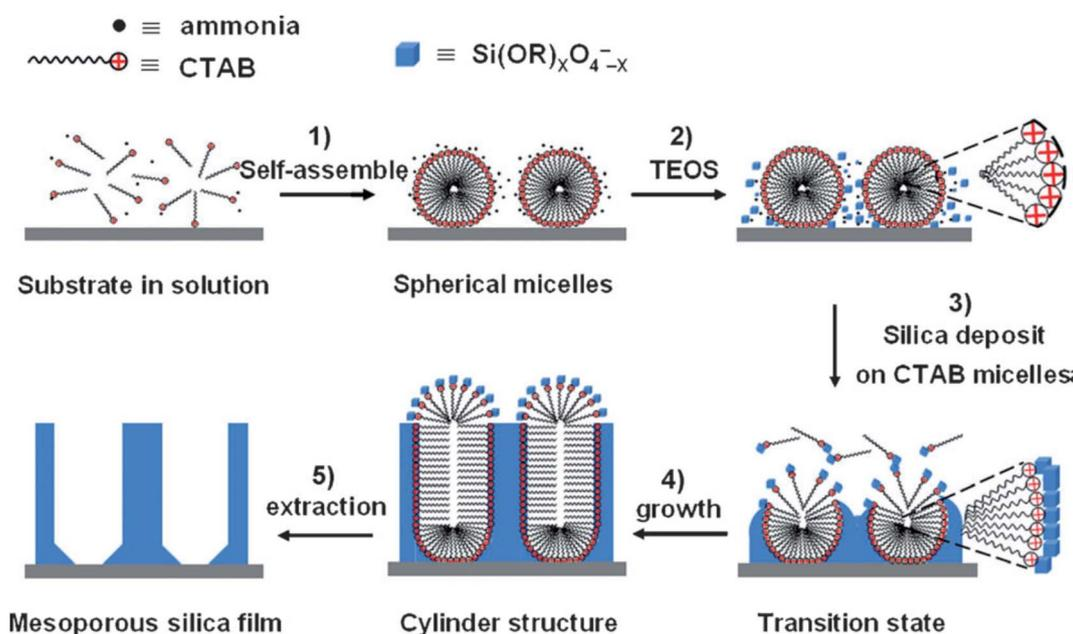
Fig. 2 Formation process of ordered mesoporous silica films with perpendicular mesochannels by the Stöber-solution spontaneous growth procedure. Reproduced with permission from ref. 36.
