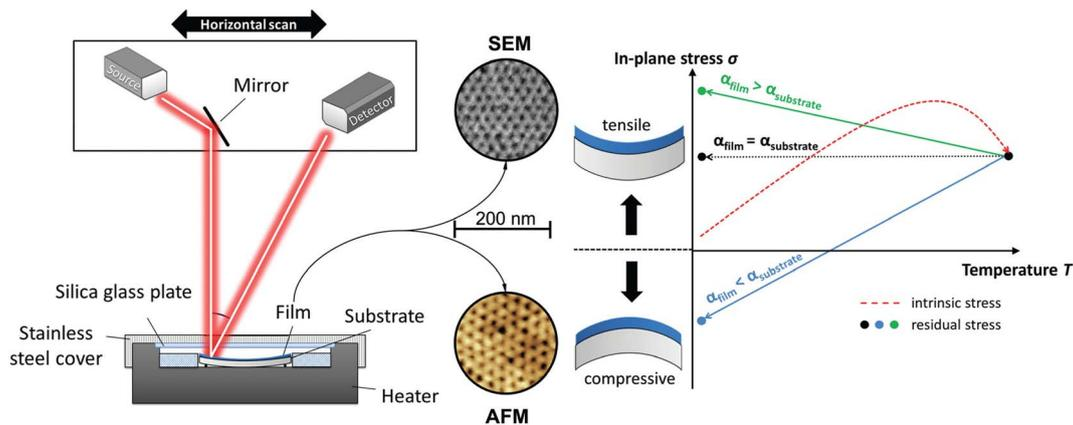
Fig. 6 (Left) Scheme of the setup of the thin film stress instrument used for curvature determination. It has a built-in heater for *in situ* measurements. (Right) Temperature dependence of the in-plane stress while heating (red dotted line) and the following natural cooling process (straight arrows). The different thermal expansion coefficients of the film and substrate directly affect the resulting residual stress. Rearranged with permission from ref. 57.
