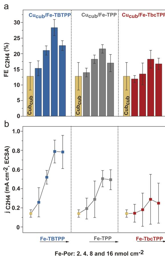
Fig. 6 (a)  $FE_{C_2H_4}$  and (b)  $j_{C_2H_4}/ECSA$  of  $Cu_{cub}/Fe-TBTPP$ ,  $Cu_{cub}/Fe-TPP$ ,  $Cu_{cub}/Fe-TbcTPP$  and  $Cu_{cub}$  at different loadings of the  $Fe-Por$  (2, 4, 8 and 16  $nmol\ cm^{-2}$ ) at  $-0.95\ V$  vs. RHE in  $CO_2$  saturated 0.1 M  $KHCO_3$  H-cell. The reported values are an average of three independent experiments with error bars indicating the standard deviations.
