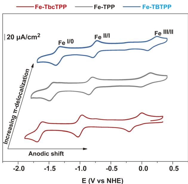
Fig. 2 Cyclic voltammetry of 0.25 mM **Fe-Por** dissolved in DMF containing 0.1 M  $\text{TBAPF}_6$  as the supporting electrolyte, carried out at a scan rate of  $100 \text{ mV s}^{-1}$ . **Fe-TbcTPP** (red), **Fe-TPP** (gray), and **Fe-TBTPP** (blue).
