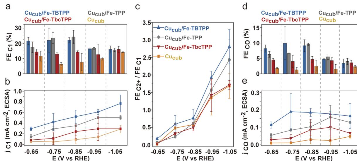
Fig. 5 (a)  $FE_{C_1}$  and (b) partial current density for the  $C_1$  products ( $j_{C_1}$ ) normalized by ECSA. (c) FE ratio of  $C_{2+}$  to  $C_1$  products. (d) FEs and (e) partial current density for CO ( $j_{CO}$ ) normalized by ECSA of  $Cu_{cub}/Fe-TBTPP$ ,  $Cu_{cub}/Fe-TPP$ ,  $Cu_{cub}/Fe-TbcTPP$  and  $Cu_{cub}$  at different potentials. The reported values are an average of three independent experiments with error bars indicating the standard deviations.
