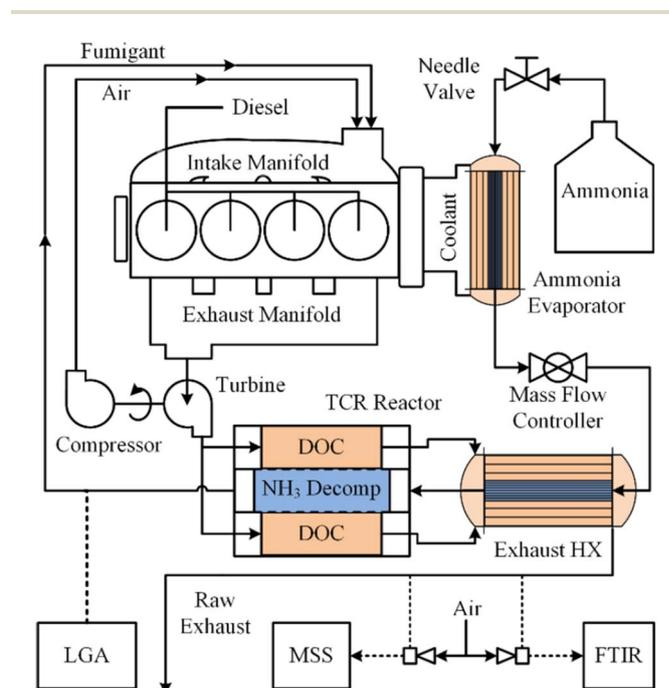
Fig. 3 On-board anhydrous  $NH_3$  thermal reforming reactor and heat exchangers for a diesel/ $NH_3$  dual-fuel tractor engine and exhaust system.<sup>13</sup> Reproduced with publisher permission from ref. 13.
