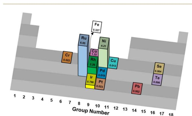
Fig. 1 Turnover frequencies (s<sup>-1</sup>) of various catalytic elements supported on Al<sub>2</sub>O<sub>3</sub> for thermal reforming of NH<sub>3</sub>.<sup>35</sup>
