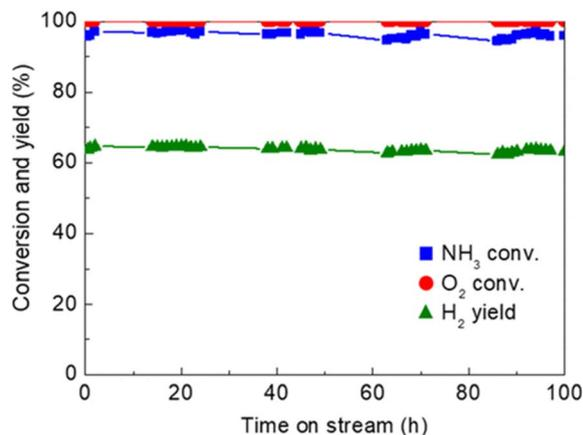
Fig. 2 Time-on-stream activity and stability of Ru/Ce<sub>0.5</sub>Zr<sub>0.5</sub>O<sub>2</sub> catalyst (1 wt% Ru loading) for oxidative reforming of NH<sub>3</sub>.<sup>85</sup> Reaction conditions: Feed rate 150 : 37.5 : 20.8 (NH<sub>3</sub> : O<sub>2</sub> : He) mL min<sup>-1</sup>, 62.5 L h<sup>-1</sup> g<sup>-1</sup> space velocity, quasi-adiabatic operation at ambient initial temperature. Reproduced with publisher permission from ref. 85.
