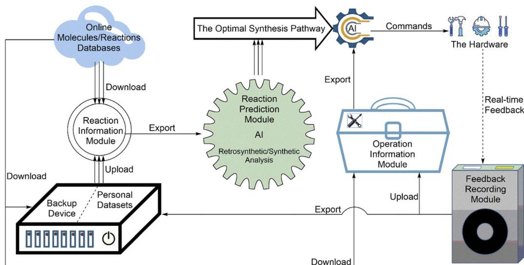
Fig. 4 The configuration of the software includes four parts: the reaction information module, reaction prediction module, reaction operation information module, and feedback recording module.
