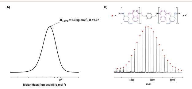
Fig. 2 (A) Molar mass distribution of poly(vinyl cyclohexene phthalate) (PvCHPE) obtained with complex 1. Conditions: [1]: [BDM]: [PA]: [vCHO] =1:4:100:2000, T=100 °C. (B) MALDI-ToF spectrum of PvCHPE obtained.  $M_{n,calc}$  (repeat unit) =272.3 g mol<sup>-1</sup>,  $M_{n,theoretical}$  (repeat unit) =27 $272.3 \text{ g mol}^{-1}$ ;  $M_{\text{n,calc}}$  (end group = BDM + K<sup>+</sup>) = 177.4 g mol<sup>-1</sup>,  $M_{\text{n,theoretical}}$  (end group) = 177.3 g mol<sup>-1</sup>.
