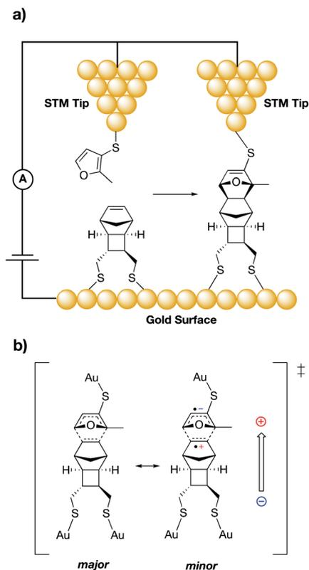
Fig. 3 (a) Experimental set-up for the Darwish, Ciampi, Diez-Perez and Coote study of the Diels–Alder reaction between an STM tip and a gold surface.<sup>27</sup> (b) Resonance structures of a proposed Diels–Alder reaction transition state; the minor resonance contributor (right) can be stabilized by a properly aligned ESF (shown with an arrow).
