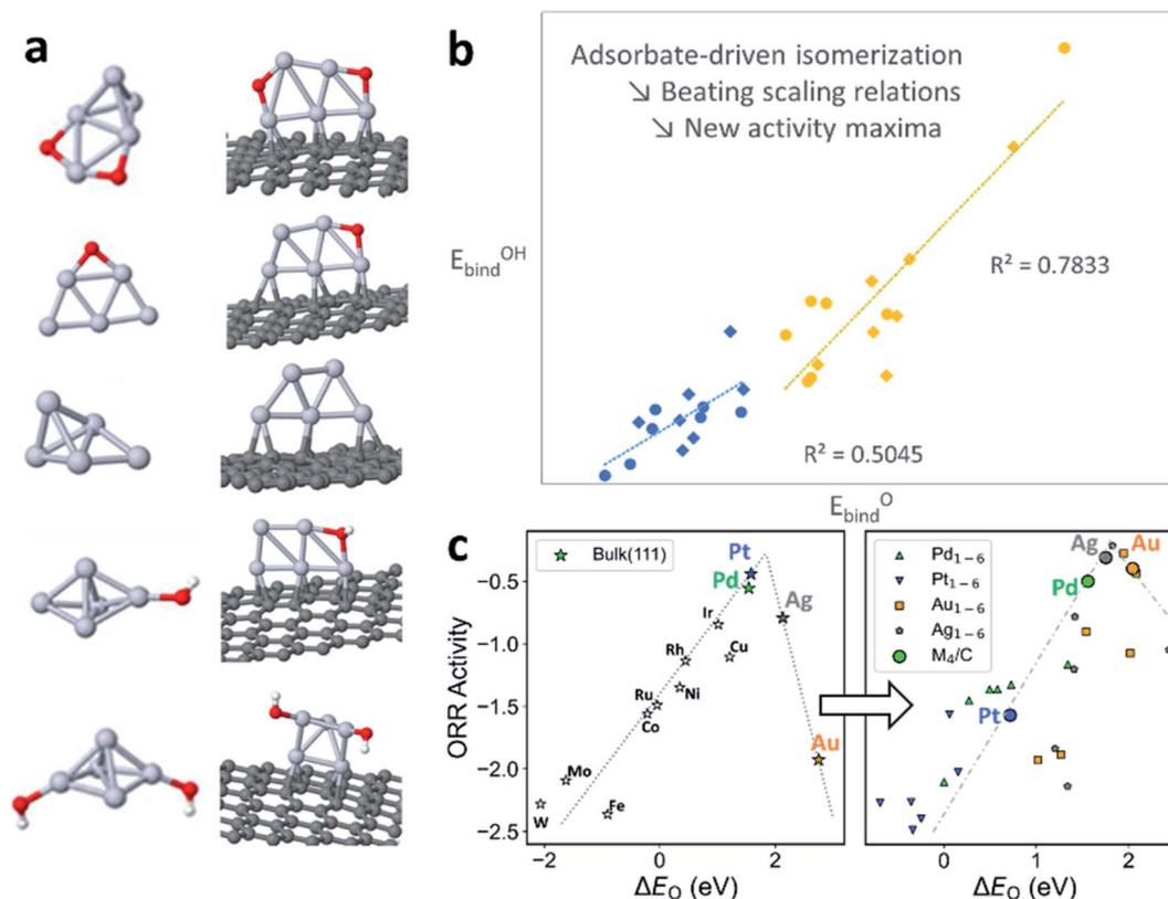
Fig. 4 (a) Changing global minima of Pt<sub>5</sub> clusters with addition of O and OH adsorbates, in both gas phase and supported on graphite. (b) The breakdown of scaling relations for ORR with Pt<sub>7</sub> clusters in gas phase and supported on graphite. PBE functional in blue, hybrid PBE0 functional in yellow. (c) Shift in the activity of metals for ORR triggered by ensembles, as shown by Sabatier volcano plots for both bulk metals and fluxional sub-nano clusters.
